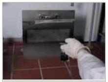
Fig. 1 Application of test soil, using a stencil
