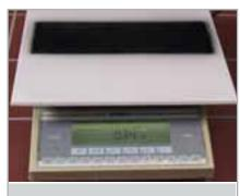
Fig. 2 Weighing of tile with test soil
