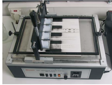
Fig.4 Test apparatus during the scrubbing process. (Source: Werner & Mertz GmbH, Mainz)
